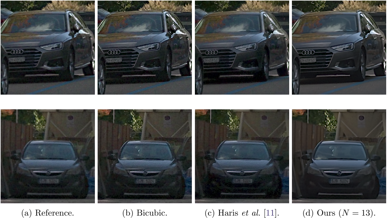
Figure 9: Comparison of different methods for \times 2 zoom on a real burst from [3]. The images are demosaiced using [10], upscaled using several methods, then postprocessed using [8]. Our pipeline manages to recover sharp details such as registration plates, while denoising even the darkest areas. Better seen by zooming on a computer screen.
