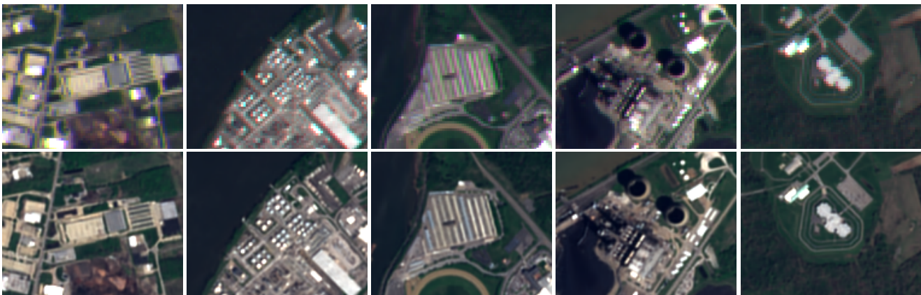
Figure 1. L1BSR produces a 5m high-resolution (HR) output with all bands correctly registered from a single 10m low-resolution (LR) Sentinel-2 L1B image with misaligned bands. Note that our method is trained on real data with self-supervision, i.e. without any ground truth HR targets.
