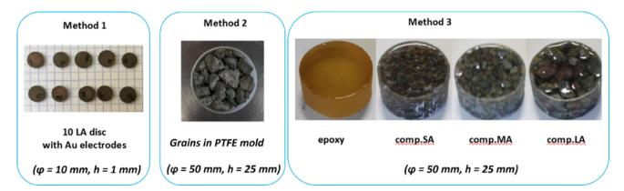
**Figure 1** Samples for the three dielectric measurements (LA, large aggregates (6-10 mm), MA, medium aggregates (4-6 mm), and SA, small aggregates (2-4 mm))
