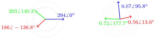
Fig. 12. Graphical representation of the arm voltages and currents found with the optimization problem for the nominal operation of the ADCC. Red, blue, and green, represent the values of the upper, middle, and lower arm respectively, in kV and kA.
