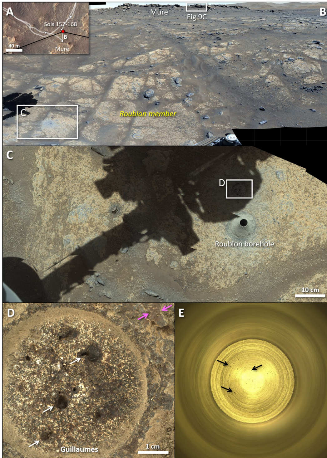
Figure 11. First abrasion at Guillaume and first sampling attempt (FTAs 22–23) at Roubion from sols 157–168. (a) Orbital context showing the extent of the image shown in (b) at the Roubion sampling location. (b) Mastcam-Z enhanced color view of the Roubion workspace in the foreground, acquired after the Guillaume abrasion, with Mure (Figure 9) in the background (sol 163, zcam08172; NASA/JPL-Caltech/ASU/MSSS/UH/F. Cary). (c) Mastcam-Z enhanced color view of the Roubion workspace after the Guillaume abrasion (d) and the Roubion target had been cored, producing a pile of drill tailings (sol 166, zcam05075; NASA/JPL-Caltech/ASU/MSSS/K. Powell). The shadow cast in both (b, c) is due to the rover's extended arm. (d) WATSON image of the Guillaume abrasion patch from 7 cm standoff, acquired on sol 160. White arrows point to irregularly shaped pits lined with dark material, and purple arrows point to a purple coating on the natural surface of the rock, exposed after dust removal by the gDRT. (e) Cachecam image of the Roubion sample tube prior to sealing, showing a mostly empty tube (diameter of 13 mm) except for several particles of martian dust (black arrows, sol 164).
