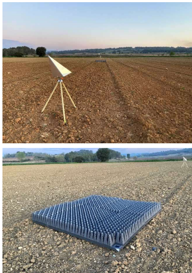
Fig. 4: Illustrations of the measurement area, trihedral and EM absorber area.
