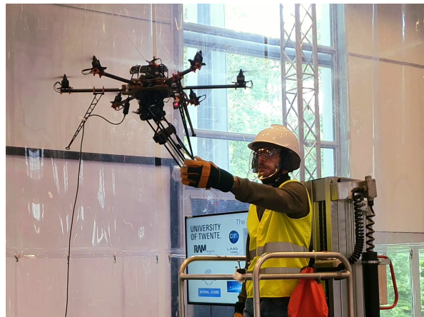
Fig. 1. Snapshot from the physical interaction experiment between the human and the AM. The human hooks a tool to the robot end effector and proceeds to reposition the aerial platform according to their preference by guiding the end effector through physical contact.
