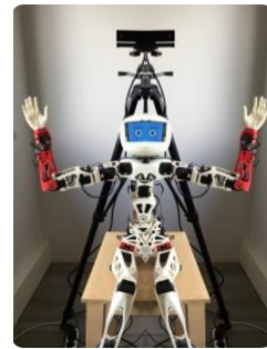
Figure 1: Setting of the system including a Microsoft Kinect v2 and an open source humanoid robot called Poppy
