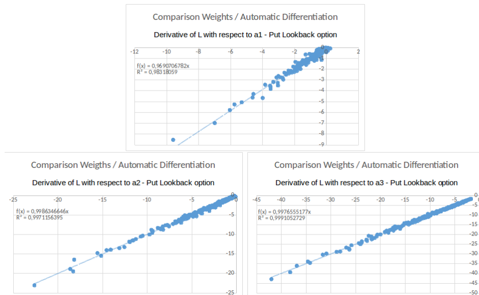
Figure 5: Results from the grid method versus results from Automatic Differentiation
