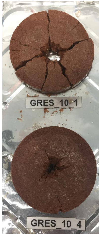
Figure 2 Impact of 1 pulse on saturated (10_1) and dry (10_4) Sandstone sample (Diameter 65mm, Height 10mm) Max voltage of pulse 90 kV, electric field 9kV/mm SELFRAG bench at BRGM
