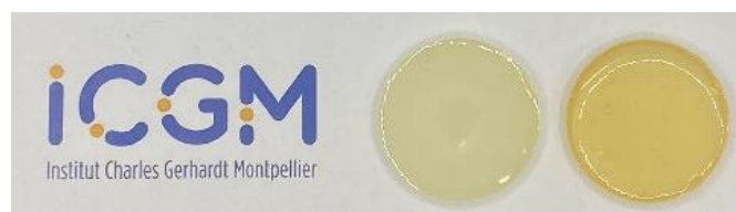
Figure 1 Picture of MDI-based thermoset (left) and BGI-based thermoset (right)
