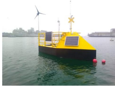
Fig. 3: Fixed beacon hosting the UWA transmission system.
