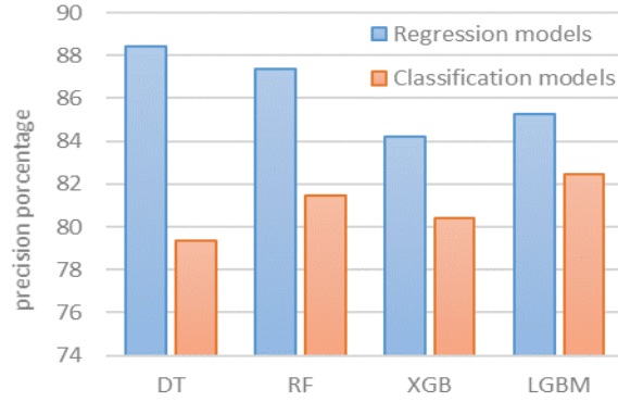
Fig. 4. Comparison between classification and regression ML models precision for ESA resistance classification problem.
