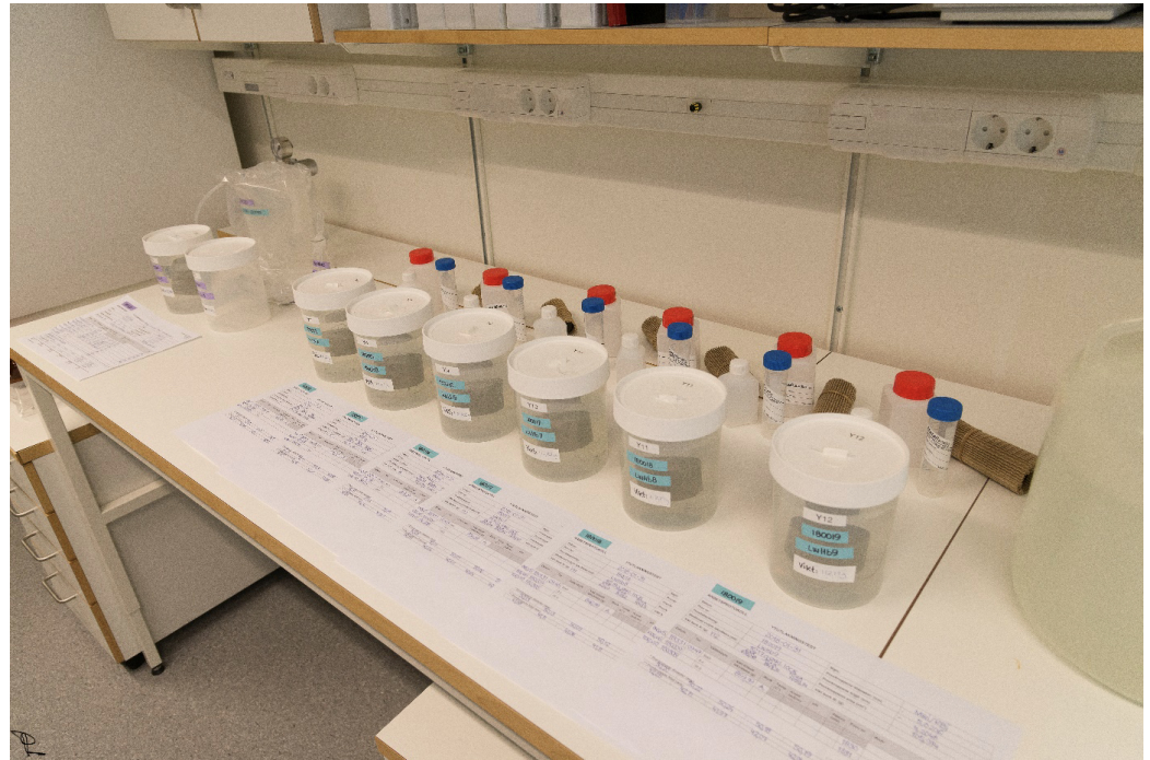
Figure 2. Process of surface leaching test on soil specimens. Photo source: Per Lindh.
