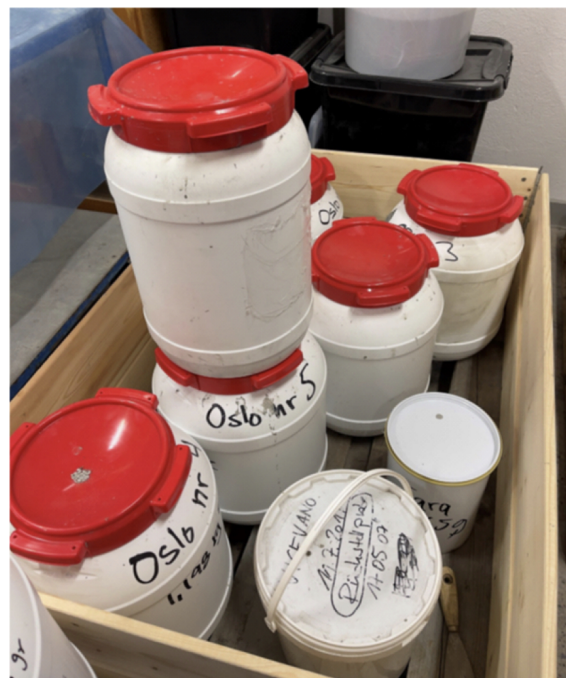
Figure 1. Containers in which dredged soil materials were stored after transportation. Photo source: Per Lindh.
