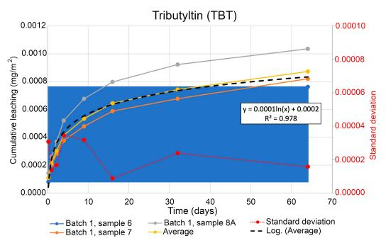
**Figure 8.** Developed leaching of TBT from the soil samples over time. Blue area represents the significant level of cumulative leaching.
