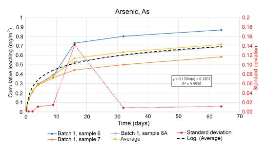
Figure 5. Cumulative leaching of arsenic (As) against time in tested specimen samples.
