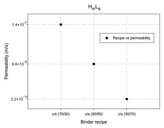
**Figure 3.** Permeability of soil in relation to the ratio between cement (c) and slag (s) for dredged soil. The best results with the lowest permeability of soil show the combination of binders for 30% cement and 70% slag. The abbreviation  $H_W L_B$  stands for "high water–low binder" level in a mixture.
