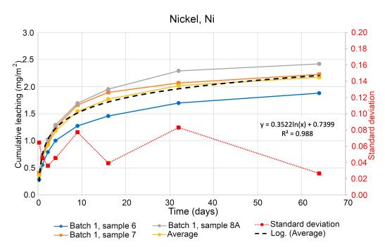
Figure 6. Cumulative leaching of nickel (Ni) over time in tested soil specimens.
