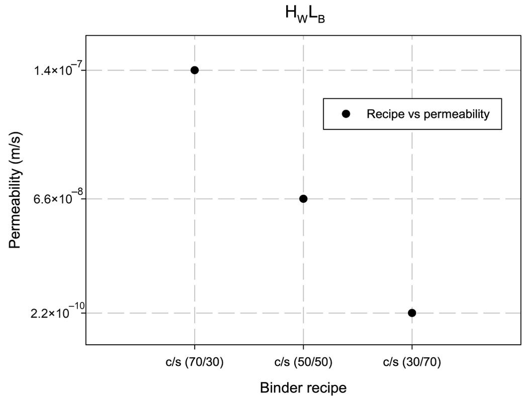
**Figure 3.** Permeability of soil in relation to the ratio between cement (c) and slag (s) for dredged soil. The best results with the lowest permeability of soil show the combination of binders for 30% cement and 70% slag. The abbreviation  $H_W L_B$  stands for “high water–low binder” level in a mixture.
