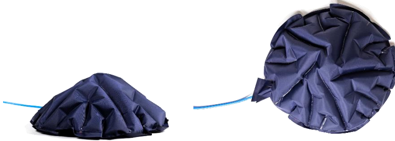
Fig. 3. Manufactured models with 2 sheets of fabric sealed according a 2D pattern.
