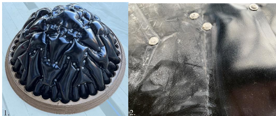
Fig. 12. Inflatable Formwork with support (1). Reusable inflatable Formwork after concrete shell fabrication (2).
