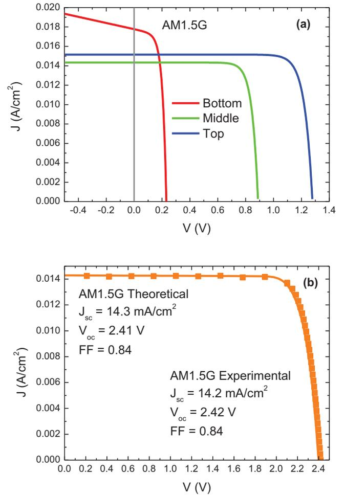
**Fig. 9.** (a)  $J(V)$  characteristics of each junction taken alone under AM1.5G, (b) comparison of the experimental (squares) and theoretical (line)  $J(V)$  characteristics of the device under AM1.5G.
