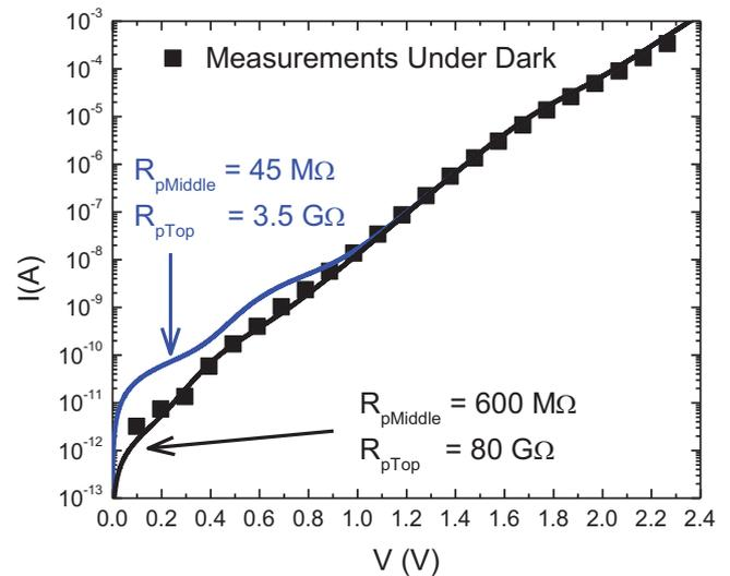
**Fig. 8.**  $I(V)$  curves under dark for our sample. Experimental results (symbol) are fitted (lines) by the results of the calculation with numerical simulations including different parameters. The arrows indicate the influences of  $R_{pTop}$  and  $R_{pMiddle}$  on the shape of the fitting curve.
