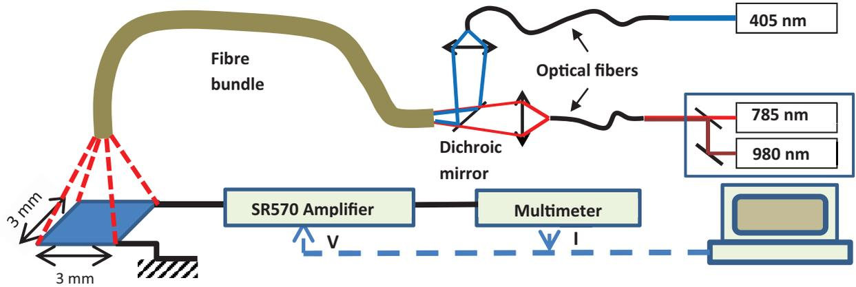
**Fig. 2.** System developed to illuminate a device with three different wavelengths. The light coming from three different lasers is injected into a fiber bundle at the other end of which the device is positioned.
