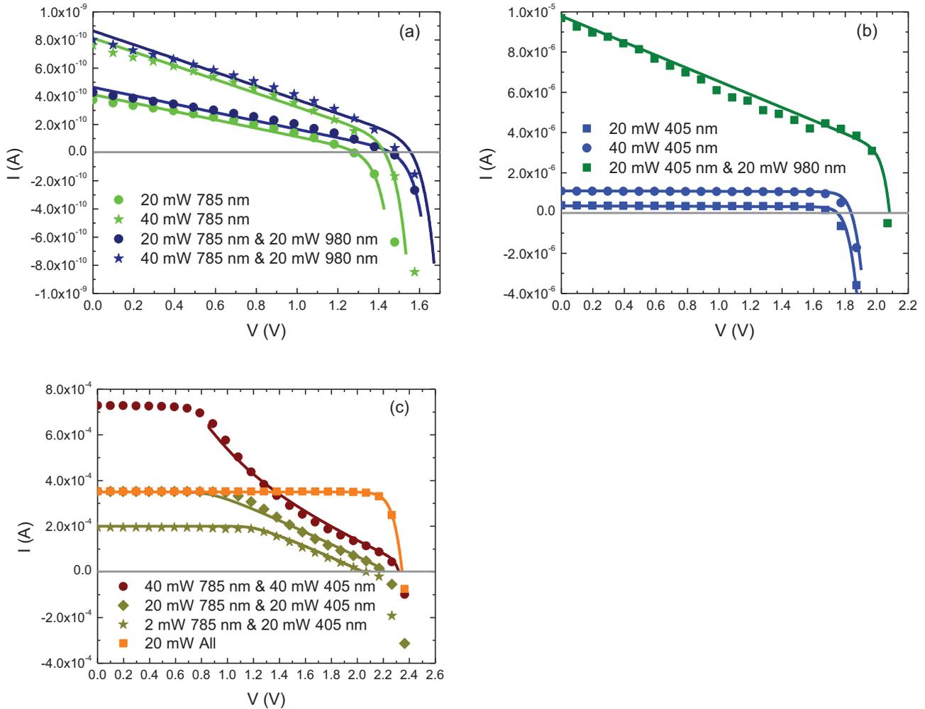
**Fig. 4.**  $I(V)$  experimental results (symbols) obtained on our sample. The power at the output of the lasers used for the experiment is displayed in the figure. The lines are the fits obtained with the numerical simulation.
