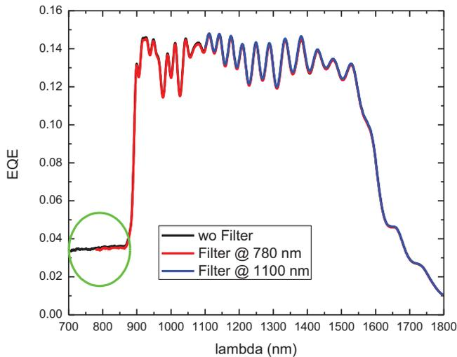
**Fig. 7.** EQE response of an isotype cell where only the bottom junction is active. In the regions where they can be measured the responses are the same independently of the used filters. The green circle indicates a contribution of the Ge cell even in the region where the light is assumed to be absorbed by the cells above.
