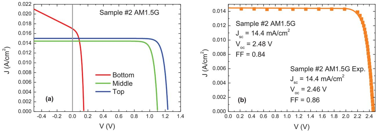
**Fig. B2.** (a)  $J(V)$  characteristics of each junction of sample #2 taken alone under AM1.5G, (b) comparison of the experimental (squares) and theoretical (line)  $J(V)$  characteristics of the device under AM1.5G.
