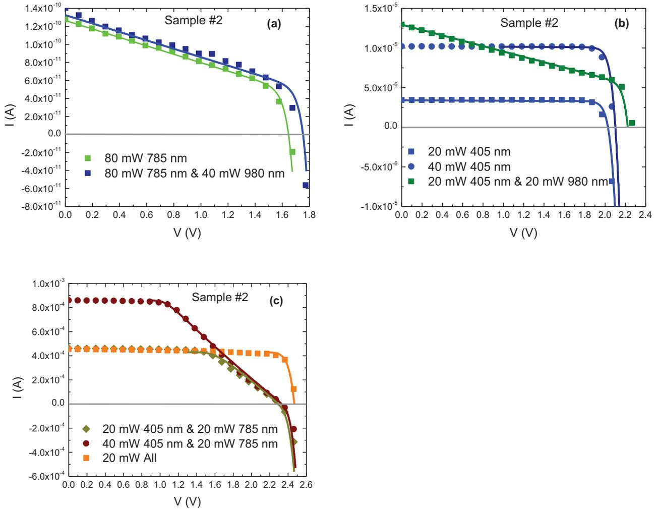
**Fig. B1.**  $I(V)$  experimental results (symbols) obtained on the second sample. The power of the lasers used for the experiment is displayed in the figure. The lines are the fits obtained with the numerical simulation.
