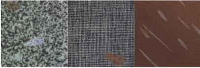
Fig. 3: Custom defective samples generated with Perin noise
