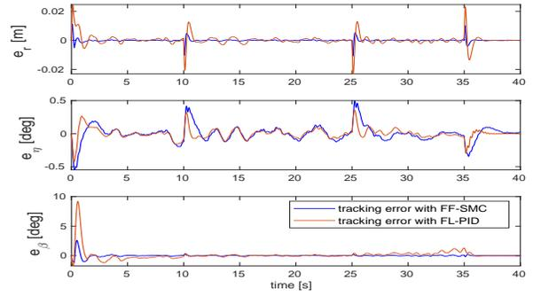
Fig. 7: Trajectory tracking errors of (FF-SMC) and (FL-PID).
