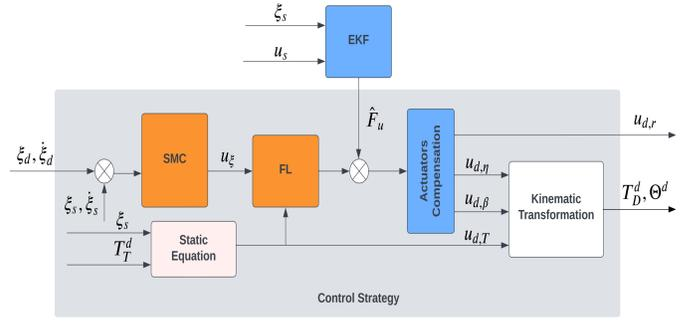
Fig. 2: Block diagram illustrating the (FF-SMC) strategy.
