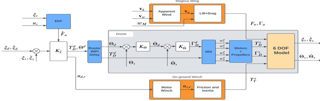
Fig. 3: Block diagram illustrating the simulation environment.
