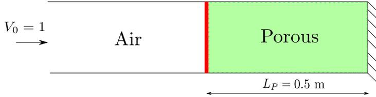
Figure 4: Illustration of the impedance tube problem
