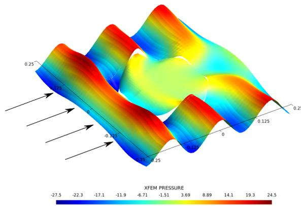
Figure 14: (a) Problem setup and mesh with refined geometric elements for a curved interface; (b) Example of real part the pressure (in Pa) under excitation of 2,000 Hz ( $p = 4$ ).
