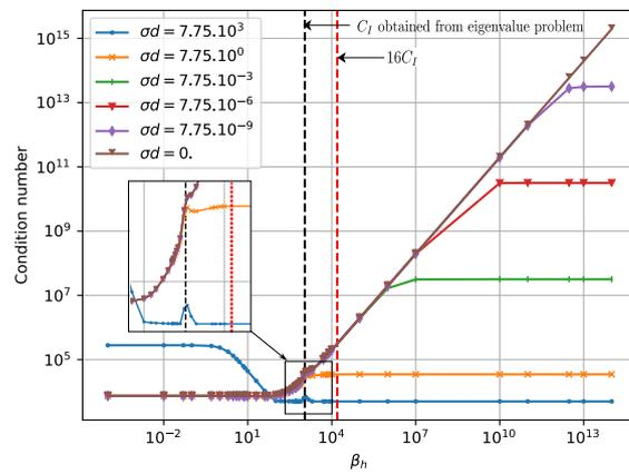
Figure 8: Sensitivity of the conditioning number w.r.t the stability parameter  $\beta_h$  ( $p = 3$ ) for different film parameters  $\sigma d$ .
