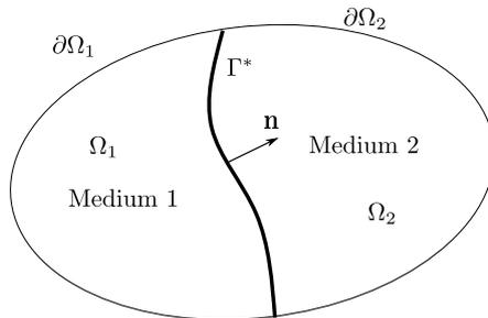
Figure 1: Two-media sound propagation configuration
