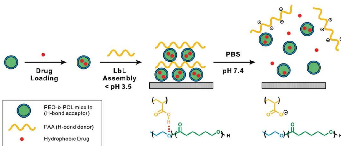
Figure 16: H-bonding layer-by-layer assembly of block copolymer micelles for triclosan delivery vehicles from surfaces. This figure has been reproduced from ref. 92 with permission from American Chemical Society, copyright 2008.
