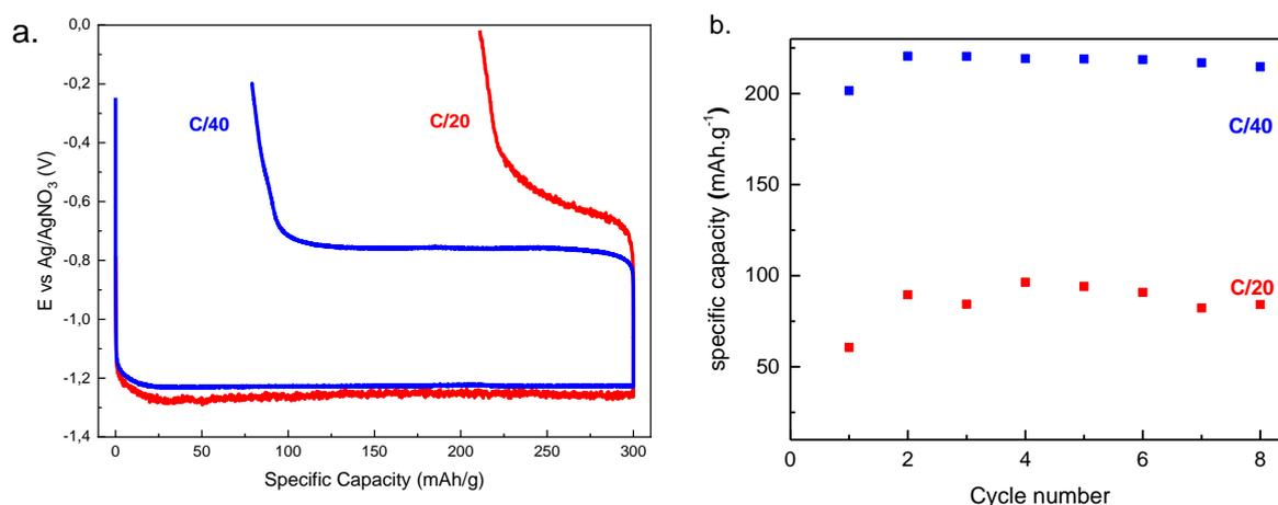
Figure 6 : Galvanostatic potential profiles at different cycling rates (a) and specific capacity as a function of the cycle number (b) on an  $AB_5$ -type alloy in the [Pyr][Ac] electrolyte.
