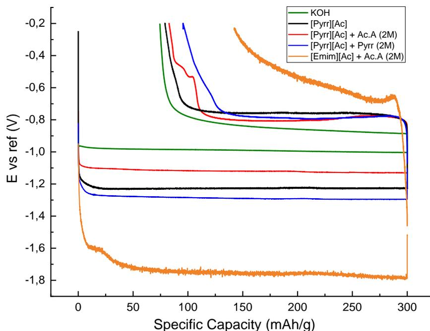
Figure 4 : Galvanostatic titration curves at the 5<sup>th</sup> cycle of AB<sub>5</sub>-type alloy in pure IL, IL/Ac.A mixture, IL/Pyrr mixture and KOH solution. Cycling performed at 25°C using C/40 rate in ILs or their mixtures and using C/10 in KOH solution, respectively.
