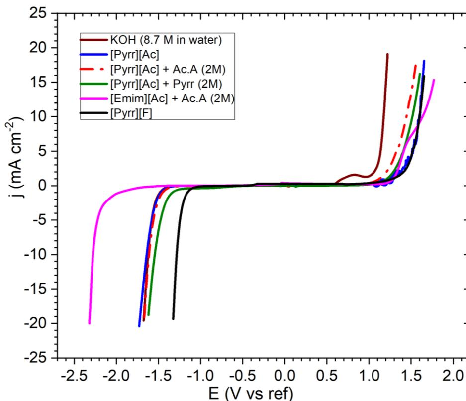
Figure 3 : LSV on gold electrode for the pure ILs and their mixtures at  $5 \text{ mV}\cdot\text{s}^{-1}$  at 298 K. The reference electrode was Hg/HgO for KOH solution and Ag/AgNO<sub>3</sub> in IL for the other systems.
