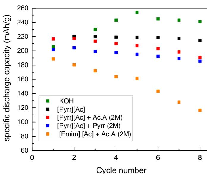
Figure 5 : Specific capacity of the material as a function of the cycle number in different electrolytes.
