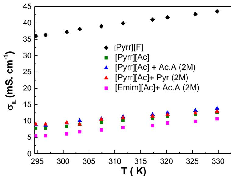
Figure 2 : Ionic conductivity measurements as a function of temperature within the range 20-60 °C for [Pyrr][F], [Pyrr][Ac], [EMIM][Ac] and [Pyrr][Ac] mixed with Ac.A or Pyr.
