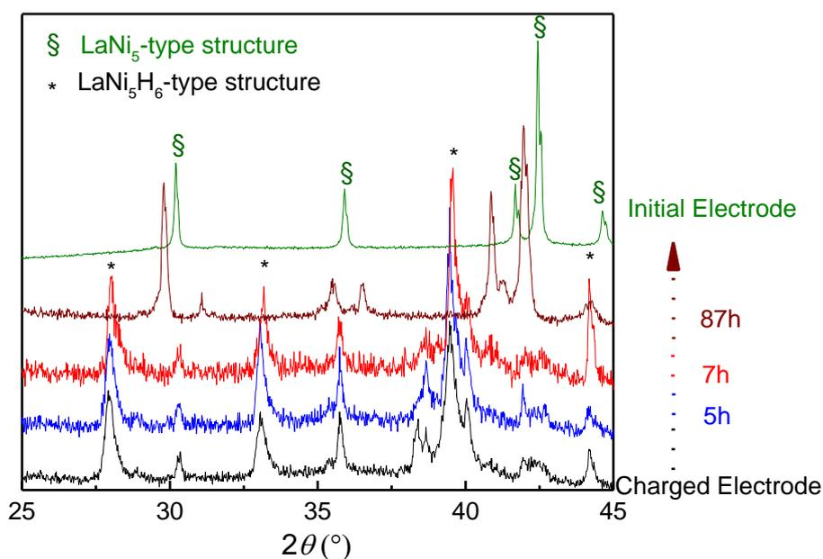
Figure 7 : XRD patterns of the initial electrode, the electrode fully charged in [Pyrr][Ac] medium and time-evolution of XRD patterns of the  $AB_5$ -type electrode during self-discharging in air. Bragg positions of  $LaNi_5$ -type structure and  $LaNi_5H_6$ -type hydride phase are indicated.
