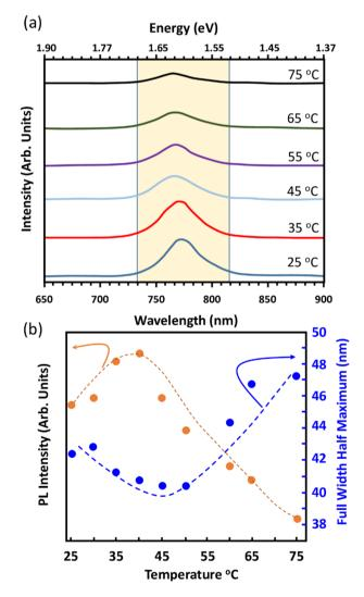
**Figure 6.** (a) Variation of the PL spectrum of the absorber perovskite films deposited on glass substrate. Measurements are performed in the range 25–75 °C. PL  $\lambda_{ext}$  = 532 nm. (b) Associated change in the PL peak intensity at ~773 nm and the FWHM as a function of temperature.
