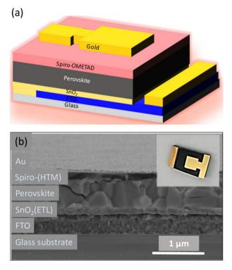
**Figure 9.** (a) Schematic diagram of the perovskite solar cell (PSC) used in this study. (b) Cross-sectional SEM image of  $Cs_{0.05}MA_{0.10}FA_{0.85}Br_{0.15}$ ) PSC. The inset shows a photograph of a PSC that is representative of those used in our experiments.
