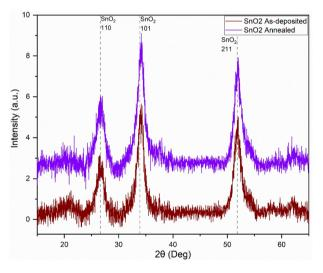
Figure 3. GIXRD for as-deposited SnO<sub>2</sub> and annealed SnO<sub>2</sub> thin film samples.
