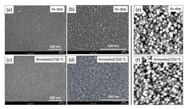
**Figure 2.** SEM (**a**–**d**) and AFM images (**e**, **f**): Top-view SEM images showing the SnO<sub>2</sub> films (**a**) as deposited magnified at x50k, (**b**) as deposited magnified at x100k, (**c**) annealed at 250 °C magnified at x50k, (**d**) annealed at 250 °C magnified at x100k; and AFM images of the SnO<sub>2</sub> films (**e**) as-deposited, (**f**) annealed at 250 °C.
