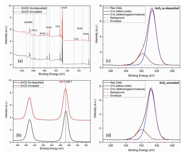
**Figure 4.** Post cleaned XPS spectra for as-deposited  $SnO_2$  and annealed  $SnO_2$  thin film samples: (**a**) surveys, (**b**) Sn3d, (**c**) O1s for as deposited  $SnO_2$ , (**d**) O1s for annealed  $SnO_2$ .
