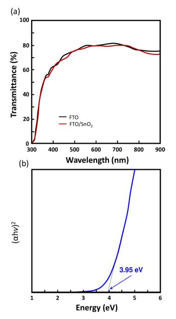
**Figure 5.** (a) Transmittance spectra % of the sputtered  $SnO_2$  film deposited on fluorine doped tin oxide (FTO) glass and FTO on glass only. (b) Associated Tauc plot showing a bandgap of 3.95 eV.
