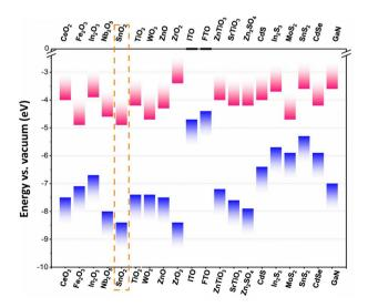
**Figure 1.** Schematic drawing showing the conduction band minimum (CBM) and the valence band maximum (VBM) of commonly employed inorganic metal materials as ETLs in PSCs<sup>29–39</sup>.
