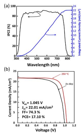
**Figure 7.** Perovskite solar cell device performance. (a) IPCE and associated integrated current density of the best device based on the sputtered  $\text{SnO}_2$  films as ETL. (b) *J*–*V* curves of the perovskite devices based on the  $\text{SnO}_2$  films as-deposited and that annealed at 250 °C (device performance results are related to the annealed  $\text{SnO}_2$  at 250 °C).
