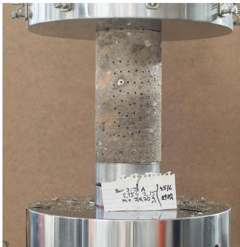
**Figure 11:** The mechanical press MTS used for UCS test. The axial resonant frequency – 4,516 Hz; flex mode resonant frequency – 2,902 Hz. Photo: Per Lindh.
