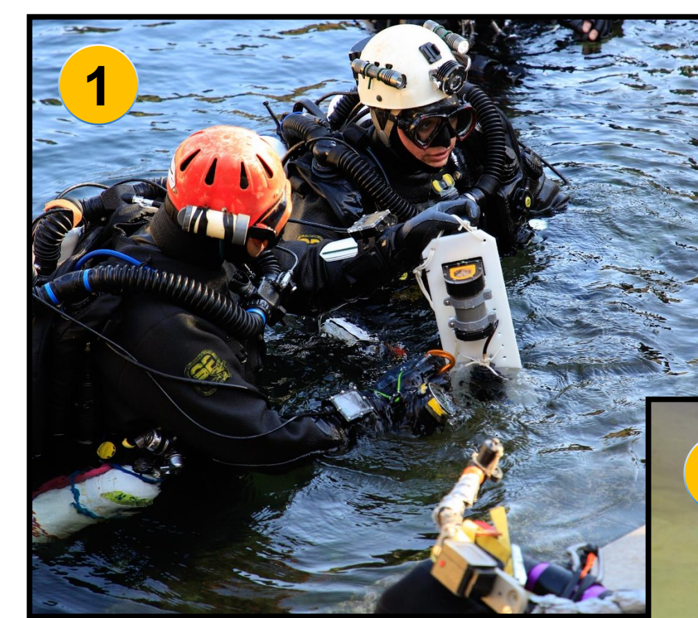
▼ TRACI: Device injecting a given volume of solution of tracer after a 30min timer (installed and activated by divers)
