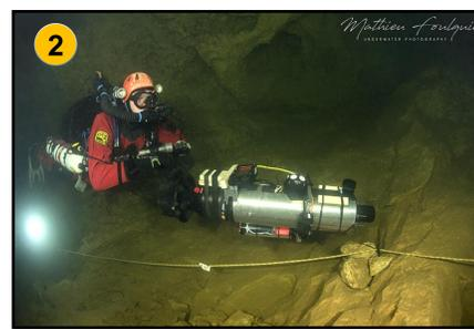
◀ NAVSCOOT: Device acquiring the 3D morphology of the conduits through acoustic resonance and measurements of the direction and velocity of its movements (guided by divers)
