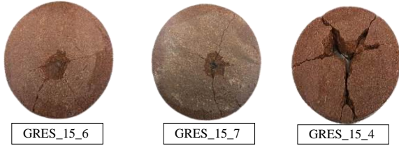
Fig. 6. Electric damage of dry sandstone under 1, 2, and 3 pulses, respectively (voltage fixed at 90 kV, electric field = 6 kV/mm)
