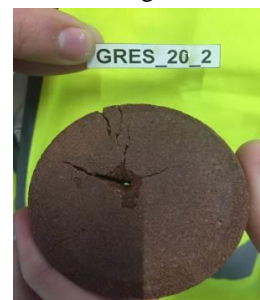
Fig. 5. Saturated sandstone with a complete channel without fragmentation after HVP treatment
