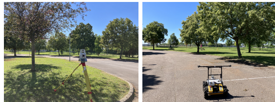
Figure 4: Illustration of the real-world experiment. Left: the Total Station scanning the area. Right: the Husky robot driving.
