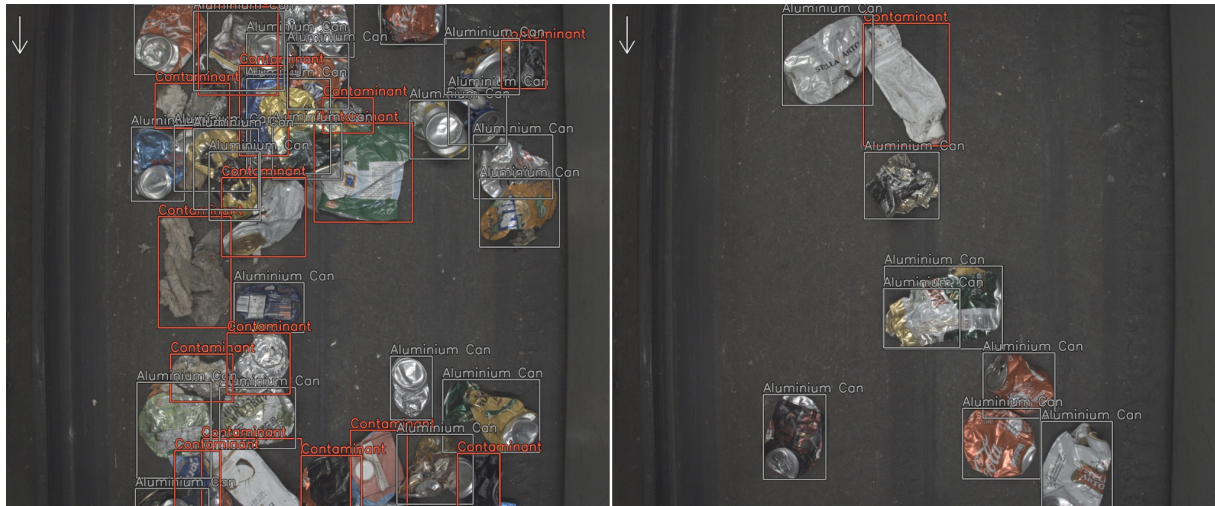
Figure 2 – Results of the object recognition on two images from the aluminium stream in an MRF. Grey boxes indicate the detections of aluminium cans and red boxes the detections of contaminants.
