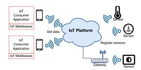
Fig. 1. IoT distributed architecture
