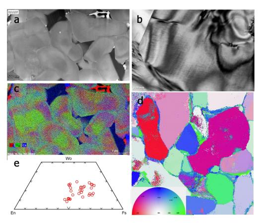
Ca-rich pyroxene (augite) often set in Ca-poor pyroxene (Ca-Mg map, Fig. 12). 159x132mm~(300~x~300~DPI)
