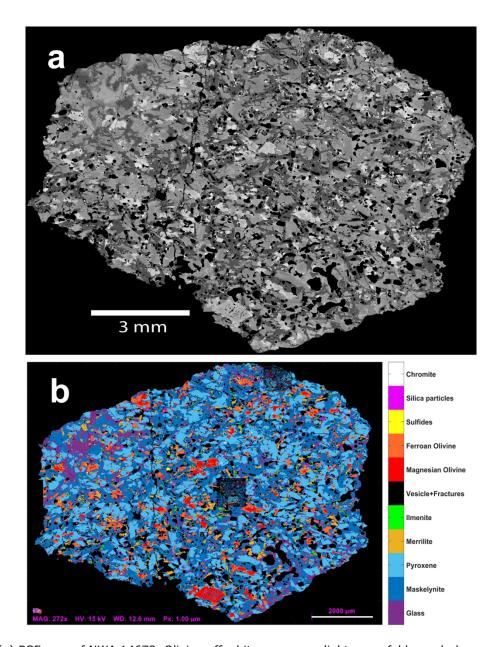
Fig. 1. (a) BSE map of NWA 14672. Olivine off-white; pyroxene light grey; feldspar dark grey; vesicles black. (b) Phase map. Olivine red-orange; pyroxene light blue. Feldspar (dark blue with vesicles black) and fine-grained components ("glass", purple) are seen throughout.
