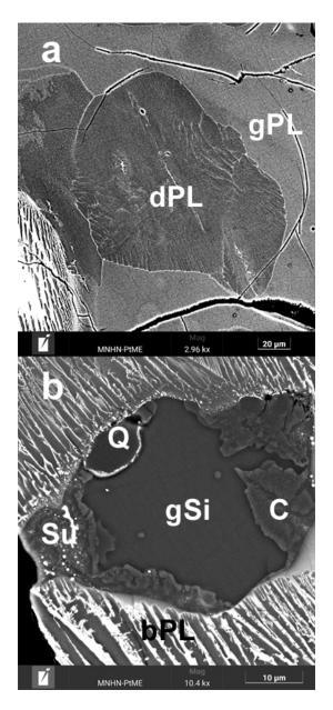
Fig. 13. (a) An aggregate of plagioclase dendrites (dPL) set in plagioclase glass (gPL). (b) Coesite (C) and quartz (Q) grown on the margins of a silica glass (gSi) particle in barred plagioclase (bPL).
