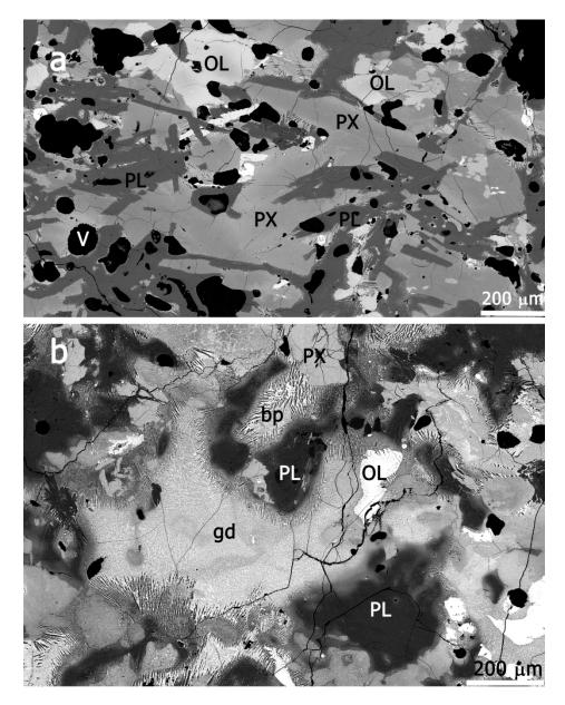
Fig. 2. BSE images. (a) Coarse-grained: vesicules (V) in plagioclase (PL), ophitic pyroxene (PX) and irregular olivine (OL). (b) Fine-grained: areas of glass with ferroan olivine dendrites (gd) and areas with feldspar bars (bp); also maskelynite/plagioclase (PL) patches, pyroxene and olivine.
