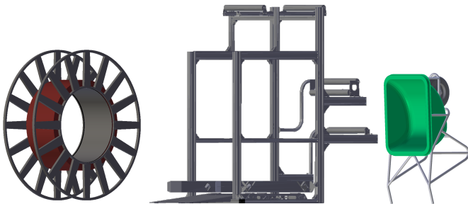
Fig. 5: 3D model of the bobbin, a simplified unwinder and a wheelbarrow. The bobbin and unwinder (real and models) are provided by an industrial partner.
