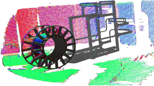
Fig. 8: Example of multi-object tracking: bobbin and unwinder. The colors illustrate the normals estimated from the captured point cloud. The grey parts correspond to the models.
