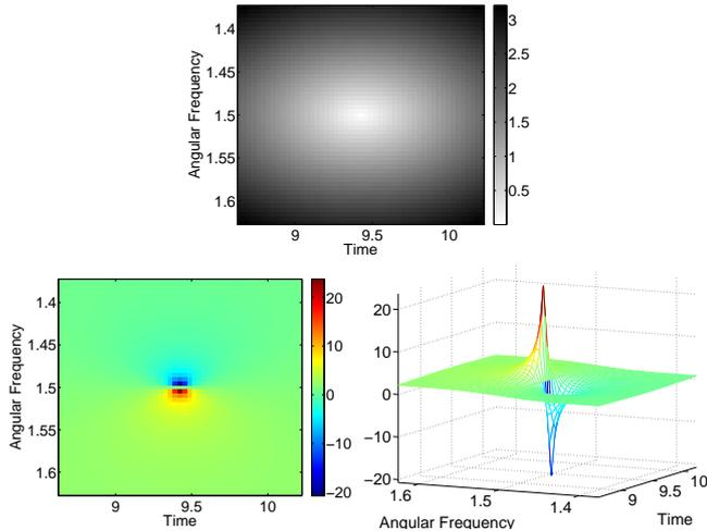
**Figure 5:** Observation for the signal defined in (9). Top: modulus of the STFT. Bottom: derivative over time of the phase of the STFT according to (11) represented as an image (left) and as a mesh (right).
