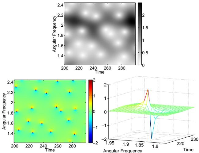
**Figure 3:** Observation for a Gaussian white noise, using a Gaussian window. Top: modulus of the STFT. Bottom-left: derivative over time of the phase of the STFT using the definition (1). Bottom-right: mesh plot of the derivative over time of the phase in the neighborhood of a zero of the STFT.
