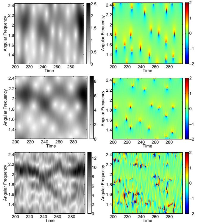
**Figure 4:** Influence of the window when analyzing a Gaussian white noise. For three different windows, on the left, modulus of the STFT, on the right, derivative over time of the phase of the STFT using the definition (1). From top to bottom, the windows are: a narrower Gaussian window, a Hamming window, a rectangular window.
