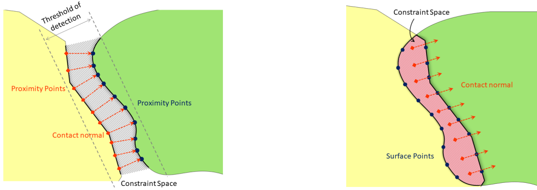
(a) For typical method of discrete collision detection, a threshold is usually used to test if the proximity points are close enough. The evaluation of potential contact normal depends directly on the surface elements (positions and normals) at the beginning of time steps.
