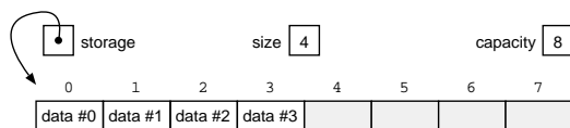
Fig. 4 Memory layout of ArrayList . Used area on the left and supply area on the right. Same indexing in the native array and in the user interface.
