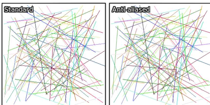
Fig. 5.2.7. Comparing traced line segments, between Brensenham's regular method and Xiaolin Wu's algorithm, implemented in the line_aa command.
