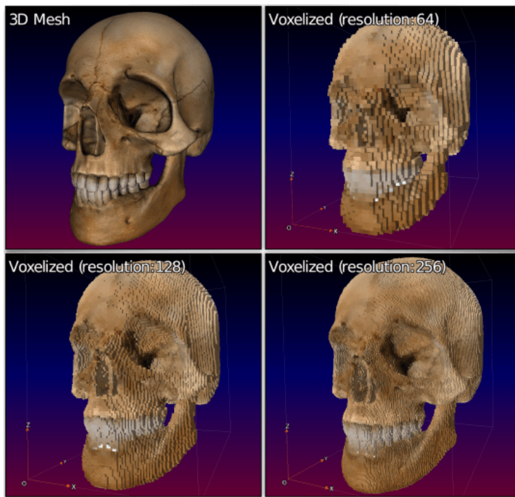
Fig. 4.2.6. Converting a textured 3D mesh to a volumetric image made of colored voxels, with the voxelize3d command.
