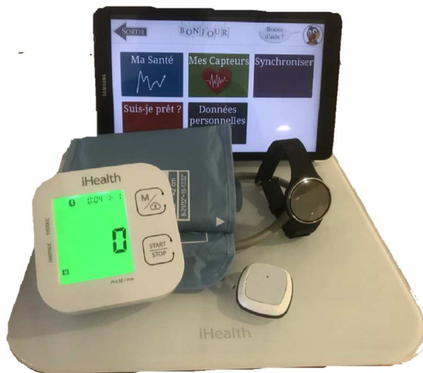
Figure 2: The ACCORDS platform including a weight scale, a tensiometer, a wrist-worn step and calories counter, an activity tracker and a tablet using the Calliopé® application.
