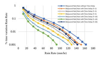
FIGURE 6. Complementary cumulative distributions of measured one-year rain rate without and with several time delays.
