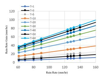
**FIGURE 7.** Measured rain rate gain  $GR_TD$  (mm/hr) versus measured rain rate  $R_{(m_{(0)_0p)})}$  (mm/hr) a function of time delays.
