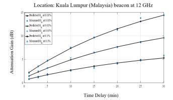
FIGURE 11. Comparison between time diversity gain measured at Kuala Lumpur with that predicted by proposed equation (24).
