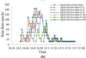
FIGURE 5. (a) An event of real time rain rate variation and (b) time delay method applied for improvement by using measured rain rate in April 29, 2014.
