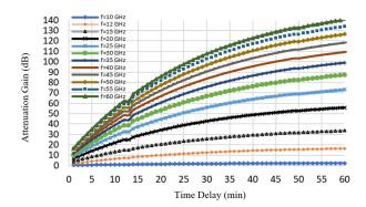
FIGURE 9. Attenuation gain obtained by marginal rain attenuation from 0 to 150 dB, at 10 to 60 GHz as the function of Time delay.
