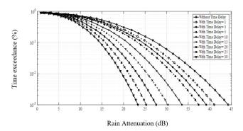
FIGURE 2. Cumulative distributions function of predicted rain attenuation with time delays by using SST.
