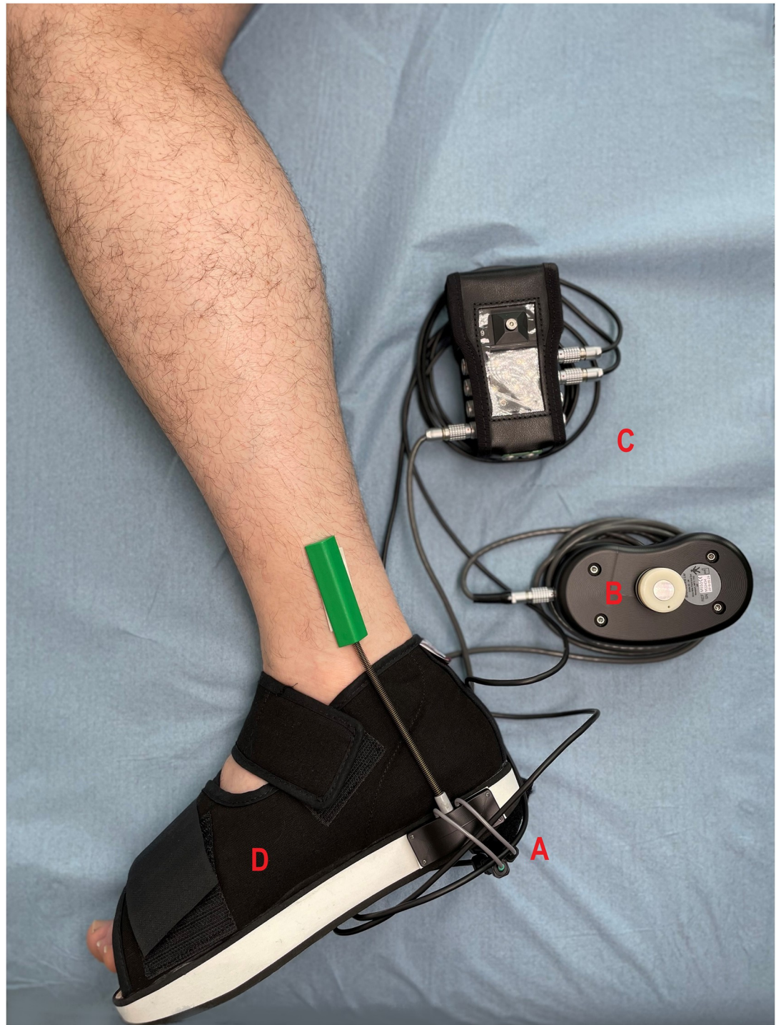
Fig 1. Equinometer with its various components: A = electronic twin-axis goniometer, B = MyoMeter electronic dynamometer, C = DataLOG and D = rigid shoe.
