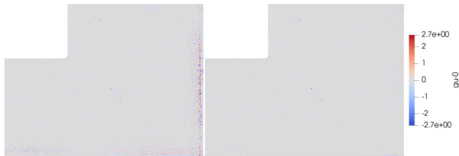
Figure 17 : Zoom on the bottom right corner of the residual map ( I_{ref} - I_{def}(u) ) in pixels at convergence of the DIC process post-buckling (left) without and (right) with geometrically non-linear elastic regularization. The improvement is clearly visible on the edge of the plate.
