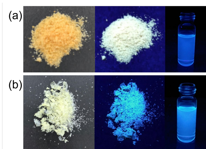
Figure 6. (a) PolyDHP in powder under visible (top-left) and UV light (top-middle) and in THF solution (1 mg/ml) under UV light (top-right), (b) btPolyDHP in powder under visible (bottom-left) and UV light (bottom-middle) and in THF solution (1 mg/ml) under UV light (bottom-right).
