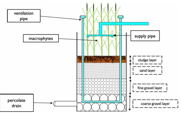
Figure 1 | Typical configuration of a PDB.
