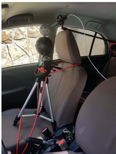
Fig. 2. Experimental setup to record 3D video and 3D audio from passenger seat viewpoint in driving situations
