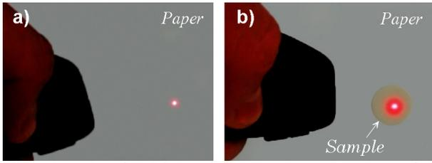
**Figure 1.** Preview of the PSF, as revealed by a laser pointer beam, of a) paper, a strongly scattering medium, and b) a circular tablet of dental composite material ("Sample") placed on top of the paper.
