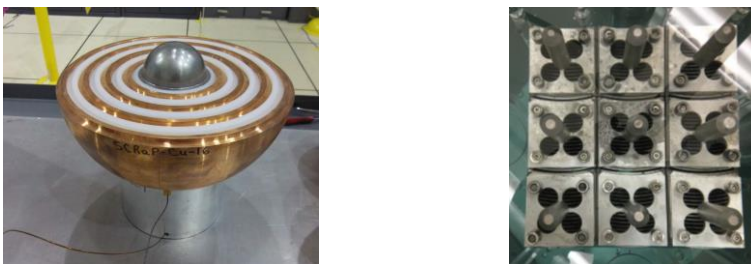
Figure 1. Left picture: SCR \alpha P benchmark during assembly, the plutonium sphere is in the center and surrounded with polyethylene (white layers) and copper (gold layers) shells. Right picture: ISSA benchmark with all available assemblies.
