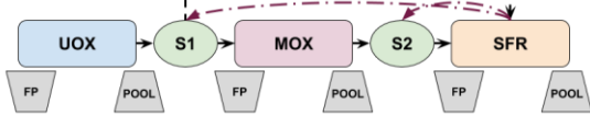
Fig 7. Schematic representation of fuel cycle facilities for the mix fleet with SFR fuel reprocessing, case B
